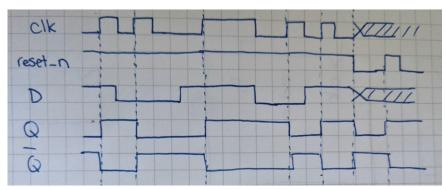
Now, I'm drawing the timing diagram of the D flip flop, with the clock at the top. Then, for each beginning of a clock cycle, I'm drawing a dotted line straight down to ensure the cycles all line up. Start with reset\_n being HIGH, and only set it to LOW further along to show that Q will follow the asynchronous reset value, and D and clk can be anything. D doesn't need to be aligned with Q and can change whenever, but Q will only change on the rising edge of a clock cycle.
