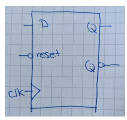
Finally, I'm writing the code. First, I'm creating the module and naming it accordingly, with the pins being D, the clock, and the Q. For example:
